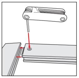
**Extrusion & Lock Connection**
