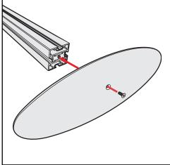
**Base Plate & Extrusion Connection**
